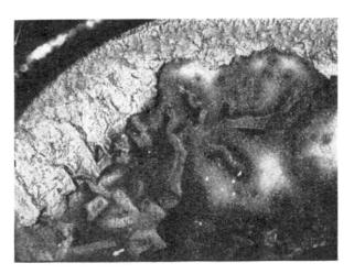
Fig. 20. Photo-micrograph of a portion of the cathode surface of a CV1070 glow-discharge tube after 2,000 hr. continuous operation at a current of 5mA.
